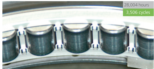
CF6-80C2, #6 bearing in D-sump
